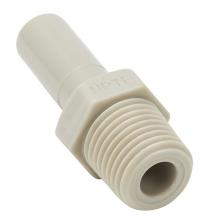
HydroMode potable water push-to-connect fitting, stem adapter, acetal body, acetal threads, (1) 3/8in plug-in to (1) 1/4in male NPT connection(s), NSF/ANSI 61. Package of 5.
