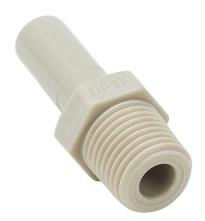
HydroMode potable water push-to-connect fitting, stem adapter, acetal body, acetal threads, (1) 3/8in plug-in to (1) 1/4in male NPT connection(s), NSF/ANSI 61. Package of 5.
