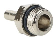
NITRA pneumatic push-to-connect fitting, stem adapter, nickel-plated brass body, 1/4in push in to 3/8in male NPT. Package of 5.
