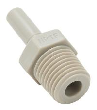
HydroMode potable water push-to-connect fitting, stem adapter, acetal body, acetal threads, (1) 1/4in plug-in to (1) 1/4in male NPT connection(s), NSF/ANSI 61. Package of 5.
