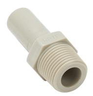
HydroMode potable water push-to-connect fitting, stem adapter, acetal body, acetal threads, (1) 1/2in plug-in to (1) 3/8in male NPT connection(s), NSF/ANSI 61. Package of 5.
