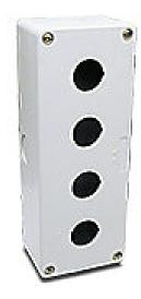
AutomationDirect pushbutton enclosure, 4 holes, 22mm, 185  $\times$  70  $\times$  51mm (HxWxD), wall mount, thermoplastic ABS, gray, screw cover
