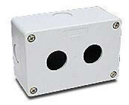
AutomationDirect pushbutton enclosure, 2 holes, 22mm, 105 x  $70 \times 51$ mm (HxWxD), wall mount, thermoplastic ABS, gray, screw cover.
