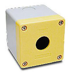
AutomationDirect pushbutton enclosure, 1 hole, 22mm, 70 x 70 x 74mm (HxWxD), wall mount, thermoplastic ABS, gray body / yellow cover, screw cover.
