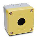
AutomationDirect pushbutton enclosure, 1 hole, 22mm, 70 x 70 x 51mm (HxWxD), wall mount, thermoplastic ABS, gray body / yellow cover, screw cover.
