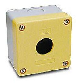
AutomationDirect pushbutton enclosure, 1 hole, 22mm,  $70 \times 70 \times 51$ mm (HxWxD), wall mount, thermoplastic ABS, gray body / yellow cover, screw cover.
