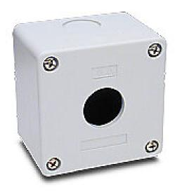
AutomationDirect pushbutton enclosure, 1 hole, 22mm,  $70 \times 70 \times 51$ mm (HxWxD), wall mount, thermoplastic ABS, gray, screw cover.
