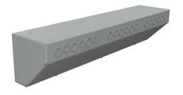
Wiegmann wiring trough, 8 x 8 x 36in (HxDxL), NEMA 1, corner mount, with knockouts, carbon steel, ANSI 61 gray, powder coat finish, screw cover.
