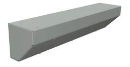
Wiegmann wiring trough, 8 x 8 x 36in (HxDxL), NEMA 1, corner mount, carbon steel, ANSI 61 gray, powder coat finish, screw cover.
