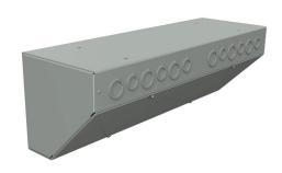
Wiegmann wiring trough, 8 x 8 x 24in (HxDxL), NEMA 1, corner mount, with knockouts, carbon steel, ANSI 61 gray, powder coat finish, screw cover.
