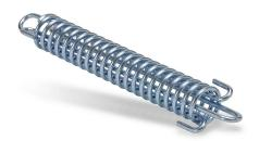
Bryant safety spring, galvanized steel, 1in diameter, 8.25in length, 80lb capacity, 850lb breaking strength, maximum deflection 3.125in at 80lbs (356N/7.94cm).
