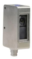
Datalogic contrast sensor, rectangular, diffuse, RGB, 6-12mm sensing distance, selectable light-on/dark-on, PNP, teach-in button, 25 kHz switching frequency, 316L stainless steel housing, 4-pin M8 quick-disconnect.
