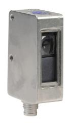
Datalogic contrast sensor, rectangular, diffuse, RGB light emission, 6-12mm sensing distance, selectable light-on/dark-on, NPN, teach-in button, 25 kHz switching frequency, 316L stainless steel housing, 4-pin M8 quick-disconnect.
