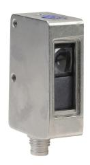
Datalogic contrast sensor, rectangular, diffuse, RGB, 6-12mm sensing distance, selectable light-on/dark-on, NPN, teach-in button, 25 kHz switching frequency, 316L stainless steel housing, 4-pin M8 quick-disconnect.
