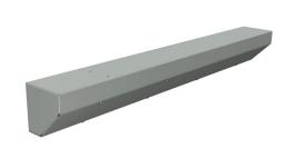
Wiegmann wiring trough, 6 x 6 x 48in (HxDxL), NEMA 1, corner mount, carbon steel, ANSI 61 gray, powder coat finish, screw cover.
