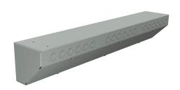
Wiegmann wiring trough, 6 x 6 x 36in (HxDxL), NEMA 1, corner mount, with knockouts, carbon steel, ANSI 61 gray, powder coat finish, screw cover.
