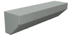
Wiegmann wiring trough, 6 x 6 x 24in (HxDxL), NEMA 1, corner mount, carbon steel, ANSI 61 gray, powder coat finish, screw cover.
