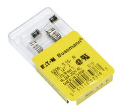
Bussmann fuse, S506 series, small dimension, time-delay, 3.15A, 250 VAC, glass tube. Package of 5. Supplemental, electronic protection applications. Manufacturer part number: S506-3.15-R.
