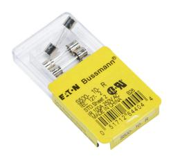
Bussmann fuse, S500 series, small dimension, fast-acting, 10A, 250 VAC, glass tube. Package of 5. Supplemental, electronic protection applications. Manufacturer part number: S500-10-R.
