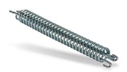
Bryant safety spring, galvanized steel, 3/4in diameter, 8.25in length, 40lb capacity, 500lb breaking strength, maximum deflection 2.75in at 40lbs (178N/6.67cm).
