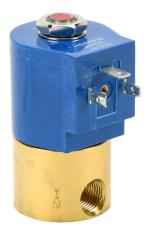
GC Valves solenoid valve, 2-port (2-way), 2-position, N.C., brass body, Viton seal(s), 1/4in female NPT inlet(s), 1/4in female NPT outlet(s), Cv=0.65, 0 psi minimum operating pressure, 24 VDC operating voltage, 18mm DIN style wiring plug.
