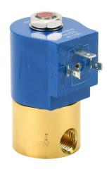
GC Valves solenoid valve, 2-port (2-way), 2-position, N.C., brass body, Viton seal(s), 1/4in female NPT inlet(s), 1/4in female NPT outlet(s), Cv=0.44, 0 psi minimum operating pressure, 24 VDC operating voltage, 18mm DIN style wiring plug.
