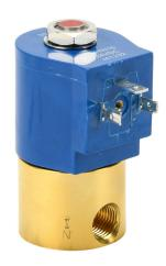
GC Valves solenoid valve, 2-port (2-way), 2-position, N.C., brass body, Viton seal(s), 1/4in female NPT inlet(s), 1/4in female NPT outlet(s), Cv=0.36, 0 psi minimum operating pressure, 24 VDC operating voltage, 18mm DIN style wiring plug.
