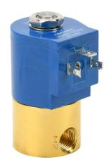
GC Valves solenoid valve, 2-port (2-way), 2-position, N.C., brass body, Viton seal(s), 1/4in female NPT inlet(s), 1/4in female NPT outlet(s), Cv=0.65, 0 psi minimum operating pressure, 120 VAC operating voltage, 18mm DIN style wiring plug.
