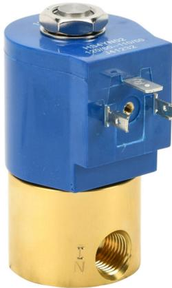
GC Valves solenoid valve, 2-port (2-way), 2-position, N.C., brass body, Viton seal(s), 1/4in female NPT inlet(s), 1/4in female NPT outlet(s), Cv=0.44, 0 psi minimum operating pressure, 120 VAC operating voltage, 18mm DIN style wiring plug.
