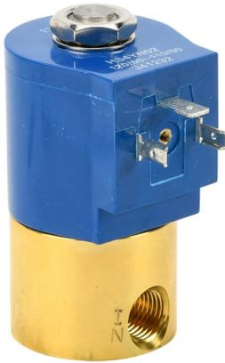
GC Valves solenoid valve, 2-port (2-way), 2-position, N.C., brass body, Viton seal(s), 1/4in female NPT inlet(s), 1/4in female NPT outlet(s), Cv=0.36, 0 psi minimum operating pressure, 120 VAC operating voltage, 18mm DIN style wiring plug.
