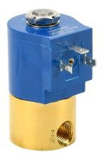
GC Valves solenoid valve, 2-port (2-way), 2-position, N.C., brass body, Viton seal(s), 1/4in female NPT inlet(s), 1/4in female NPT outlet(s), Cv=0.36, 0 psi minimum operating pressure, 120 VAC operating voltage, 18mm DIN style wiring plug.
