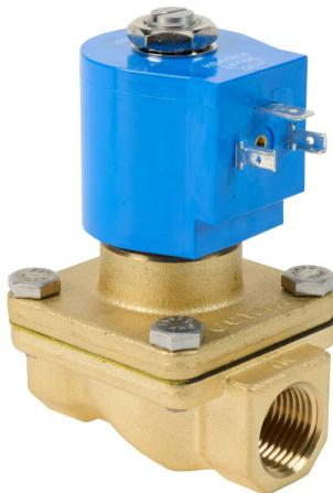
GC Valves solenoid valve, 2-port (2-way), 2-position, N.C., brass body, Viton seal(s), 1/2in female NPT inlet(s), 1/2in female NPT outlet(s), Cv=4.3, 4 psi minimum operating pressure, 24 VDC operating voltage, 18mm DIN style wiring plug.
