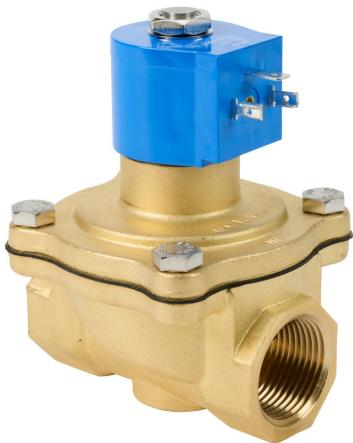
GC Valves solenoid valve, 2-port (2-way), 2-position, N.C., brass body, nitrile seal(s), 1in female NPT inlet(s), 1in female NPT outlet(s), Cv=13, 5 psi minimum operating pressure, 24 VDC operating voltage, 18mm DIN style wiring plug.
