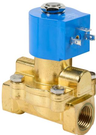
GC Valves solenoid valve, 2-port (2-way), 2-position, N.C., brass body, Viton seal(s), 1/2in female NPT inlet(s), 1/2in female NPT outlet(s), Cv=3.3, 1 psi minimum operating pressure, 24 VDC operating voltage, 18mm DIN style wiring plug.
