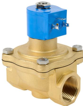
GC Valves solenoid valve, 2-port (2-way), 2-position, N.C., brass body, Viton seal(s), 1in female NPT inlet(s), 1in female NPT outlet(s), Cv=13, 5 psi minimum operating pressure, 120 VAC operating voltage, 18mm DIN style wiring plug.
