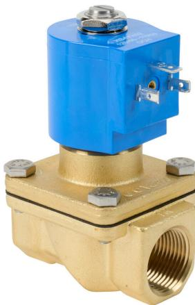
GC Valves solenoid valve, 2-port (2-way), 2-position, N.C., brass body, Viton seal(s), 3/4in female NPT inlet(s), 3/4in female NPT outlet(s), Cv=6.7, 4 psi minimum operating pressure, 120 VAC operating voltage, 18mm DIN style wiring plug.
