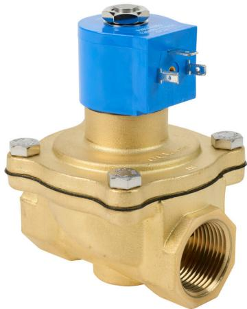
GC Valves solenoid valve, 2-port (2-way), 2-position, N.C., brass body, nitrile seal(s), 1in female NPT inlet(s), 1in female NPT outlet(s), Cv=13, 5 psi minimum operating pressure, 120 VAC operating voltage, 18mm DIN style wiring plug.
