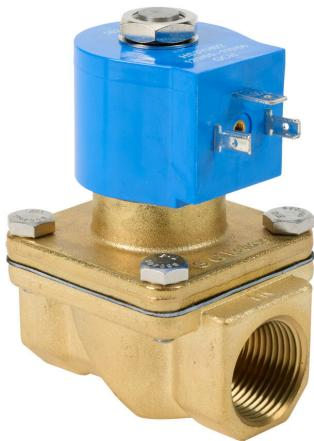
GC Valves solenoid valve, 2-port (2-way), 2-position, N.C., brass body, nitrile seal(s), 3/4in female NPT inlet(s), 3/4in female NPT outlet(s), Cv=6.7, 4 psi minimum operating pressure, 120 VAC operating voltage, 18mm DIN style wiring plug.
