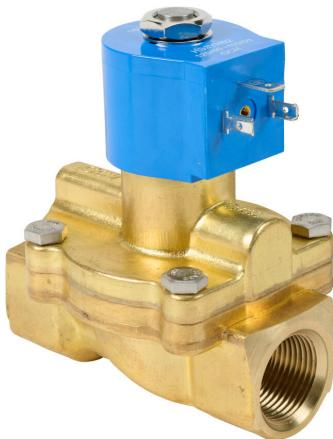
GC Valves solenoid valve, 2-port (2-way), 2-position, N.C., brass body, Viton seal(s), 3/4in female NPT inlet(s), 3/4in female NPT outlet(s), Cv=6.1, 1 psi minimum operating pressure, 120 VAC operating voltage, 18mm DIN style wiring plug.
