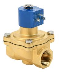
GC Valves solenoid valve, 2-port (2-way), 2-position, N.C., brass body, Viton seal(s), 1in female NPT inlet(s), 1in female NPT outlet(s), Cv=13, 5 psi minimum operating pressure, 24 VDC operating voltage, 18mm DIN style wiring plug.
