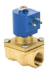
GC Valves solenoid valve, 2-port (2-way), 2-position, N.C., brass body, Viton seal(s), 3/4in female NPT inlet(s), 3/4in female NPT outlet(s), Cv=6.7, 4 psi minimum operating pressure, 24 VDC operating voltage, 18mm DIN style wiring plug.
