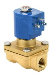
GC Valves solenoid valve, 2-port (2-way), 2-position, N.C., brass body, Viton seal(s), 3/8in female NPT inlet(s), 3/8in female NPT outlet(s), Cv=4.3, 4 psi minimum operating pressure, 24 VDC operating voltage, 18mm DIN style wiring plug.
