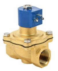
GC Valves solenoid valve, 2-port (2-way), 2-position, N.C., brass body, nitrile seal(s), 1in female NPT inlet(s), 1in female NPT outlet(s), Cv=13, 5 psi minimum operating pressure, 24 VDC operating voltage, 18mm DIN style wiring plug.
