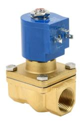
GC Valves solenoid valve, 2-port (2-way), 2-position, N.C., brass body, nitrile seal(s), 3/4in female NPT inlet(s), 3/4in female NPT outlet(s), Cv=6.7, 4 psi minimum operating pressure, 24 VDC operating voltage, 18mm DIN style wiring plug.
