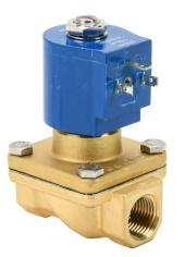
GC Valves solenoid valve, 2-port (2-way), 2-position, N.C., brass body, nitrile seal(s), 1/2in female NPT inlet(s), 1/2in female NPT outlet(s), Cv=4.3, 4 psi minimum operating pressure, 24 VDC operating voltage, 18mm DIN style wiring plug.
