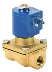
GC Valves solenoid valve, 2-port (2-way), 2-position, N.C., brass body, nitrile seal(s), 3/8in female NPT inlet(s), 3/8in female NPT outlet(s), Cv=4.3, 4 psi minimum operating pressure, 24 VDC operating voltage, 18mm DIN style wiring plug.
