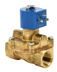
GC Valves solenoid valve, 2-port (2-way), 2-position, N.C., brass body, Viton seal(s), 3/4in female NPT inlet(s), 3/4in female NPT outlet(s), Cv=6.1, 1 psi minimum operating pressure, 24 VDC operating voltage, 18mm DIN style wiring plug.
