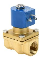
GC Valves solenoid valve, 2-port (2-way), 2-position, N.C., brass body, Viton seal(s), 3/4in female NPT inlet(s), 3/4in female NPT outlet(s), Cv=6.7, 4 psi minimum operating pressure, 120 VAC operating voltage, 18mm DIN style wiring plug.
