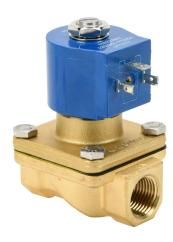
GC Valves solenoid valve, 2-port (2-way), 2-position, N.C., brass body, Viton seal(s), 1/2in female NPT inlet(s), 1/2in female NPT outlet(s), Cv=4.3, 4 psi minimum operating pressure, 120 VAC operating voltage, 18mm DIN style wiring plug.
