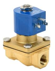
GC Valves solenoid valve, 2-port (2-way), 2-position, N.C., brass body, Viton seal(s), 3/8in female NPT inlet(s), 3/8in female NPT outlet(s), Cv=4.3, 4 psi minimum operating pressure, 120 VAC operating voltage, 18mm DIN style wiring plug.
