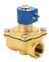
GC Valves solenoid valve, 2-port (2-way), 2-position, N.C., brass body, nitrile seal(s), 1in female NPT inlet(s), 1in female NPT outlet(s), Cv=13, 5 psi minimum operating pressure, 120 VAC operating voltage, 18mm DIN style wiring plug.
