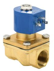
GC Valves solenoid valve, 2-port (2-way), 2-position, N.C., brass body, nitrile seal(s), 3/4in female NPT inlet(s), 3/4in female NPT outlet(s), Cv=6.7, 4 psi minimum operating pressure, 120 VAC operating voltage, 18mm DIN style wiring plug.
