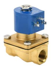
GC Valves solenoid valve, 2-port (2-way), 2-position, N.C., brass body, nitrile seal(s), 1/2in female NPT inlet(s), 1/2in female NPT outlet(s), Cv=4.3, 4 psi minimum operating pressure, 120 VAC operating voltage, 18mm DIN style wiring plug.
