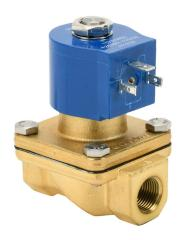
GC Valves solenoid valve, 2-port (2-way), 2-position, N.C., brass body, nitrile seal(s), 3/8in female NPT inlet(s), 3/8in female NPT outlet(s), Cv=4.3, 4 psi minimum operating pressure, 120 VAC operating voltage, 18mm DIN style wiring plug.
